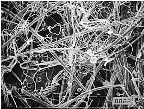
Figure 11 SEM analysis picture of fracture region from tensile test of SRIM composite containing epoxide-treated p -aramid fiber. Original picture 200 \times .
